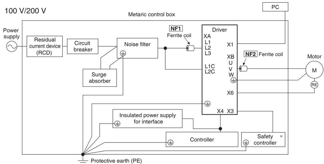
For [NF1] to [NF2], refer to the Table "Ferrite coil" (P.2-5).
