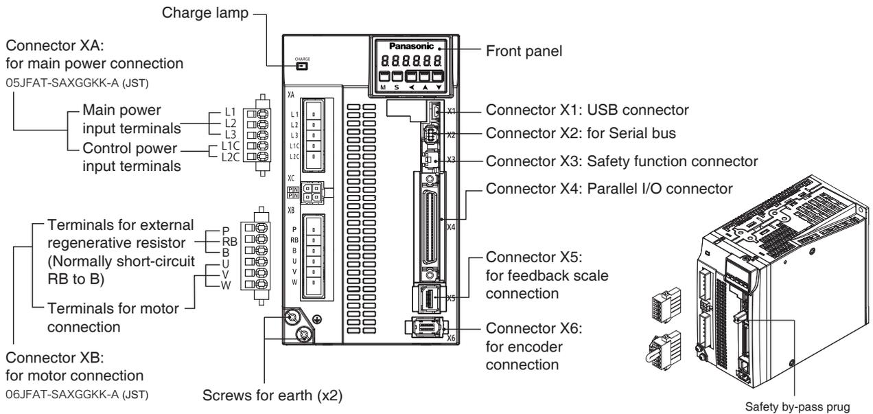
**Note** • Connector XA and XB are attached in A to D-frame driver.
