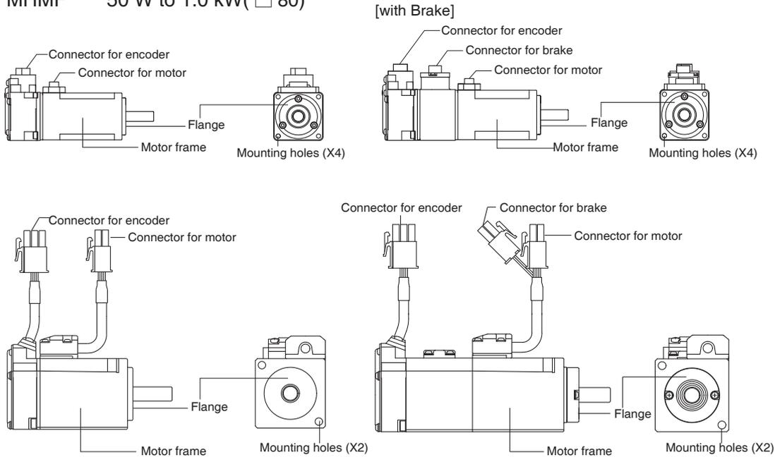
e.g.) : Low inertia type (MSMF series, 50 W), High inertia type (MHMF series, 50 W)
